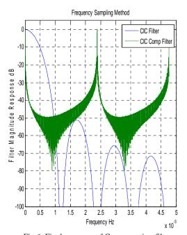
Fig 6. Final response of Compensation filter From figure 5, It can be seen, the new design of filter spectral characteristics has been significantly improved, increasing the stop band attenuation, and transition zone is more sharp, better able to reject the image aliasing. In addition, from Figures 5 and 6 can also be seen through the sidelobe suppression also of compensated CIC filter meet.
