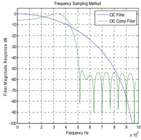
Fig 5- Response of CIC compensation filter
