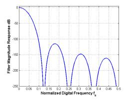
Figure .2 Magnitude Response of a CIC Filter with N = 9, R = 8, and M = 1
